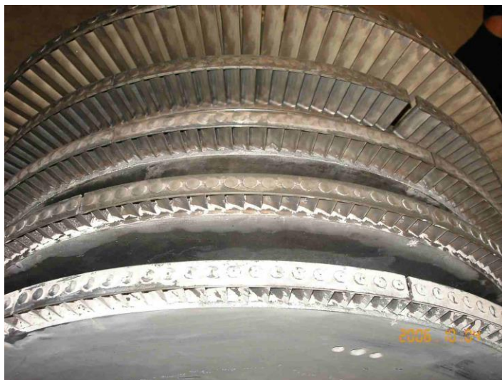
Figure 42 Turbine Blade Fouling
