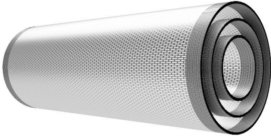
Figure 10 Containment chamber without ringlet in place
